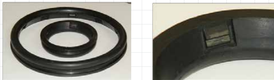
Fig. 2.10.11: Modified gaskets with steel inserts
